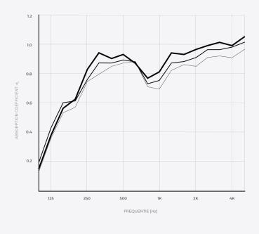
Distance of 200mm from the wall. 9mm 12mm 24mm
